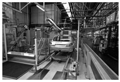
Peugeot assembly line. In this assembly line, each workstation is designed to perform a specific process. Thus, the car is constructed as it moves down the line and ultimately emerges as a finished product. Alamy Images
